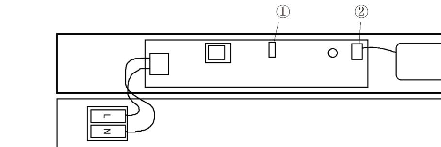
1. Remove 2-PIN connector for Non-Maintained Operation
